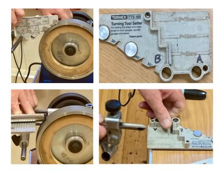
The Tormek angle setter – or similar on other set ups – is the best tool for setting precise angles but, once you've established set up, you should consider making your own jig such as the one shown below. This will give consistent repeatability and save time.
