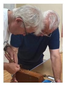
The Tormek "Tool Setter" jig being used to set desired grind angles
